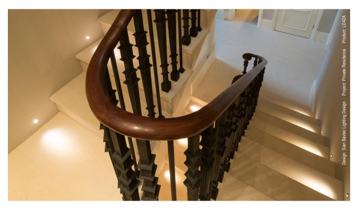
LD42 is a miniature recessed LED wall light, ideal for discreet lighting of steps and pathways. It is a high quality fitting that can be used for interior or exterior applications, including yachts. Low glare is achieved by a recessed lens assembly set back into a black anodised body. Optional half moon glare shield and 20° tilt film further reduce glare.
